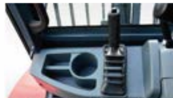
Ratchet type hand brake is reliable and has low operating force.
