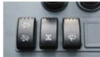
Equipped with two wheel drive/four wheel drive switching function, two wheel drive and four wheel drive can be switched at any time. It is convenient.
