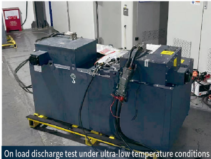
On load discharge test under ultra-low temperature conditions
