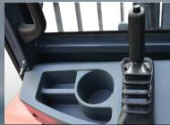
Ratchet type hand brake, reliable movement, small operating force
